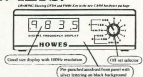
The HOWES DFD4 is an add-on Digital Readout for analogue receivers and transceivers. If you have an FRG7, an analogue FT101 or a similar type of rig, then the DFD4 has been designed with you in mind. The DFD4 is a frequency counter that can be programmed for any IF offset so it can be used with almost any radio, including the old Government surplus sets. It can also count down as well as up, so it is suitable for "reverse tuning" rigs too.
